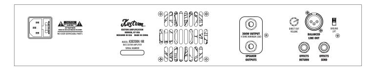
**Speaker Outputs:** These are two-conductor, ¼-inch external speaker jacks. These jacks are wired in a parallel configuration. Use them to connect the amplifier head to speaker cabinets with a minimum total impedance of 4 ohms. (**Note:** Be sure that the amp is turned off before connecting or disconnecting speaker cabinets.) *Examples:*
